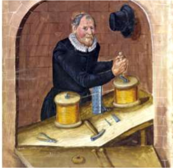
Figure 3. Drawing wire through a die fixed on a table, Nuremberg, 1625 (Hausbuch 1625)
